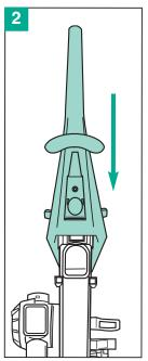
Slide handle onto vacuum back and push down until it snaps.
